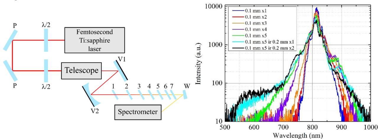
Fig. 1. In a left side: experimental setup: P – polarizer, V1 – flat mirror, V2 – concave mirror ( $f=750\text{mm}$ ), 1, 2, 3 and so on – thin plates, W – wedge. In a right side: radiation spectra after each plate (plates order in experimental setup are placed in the same order as written).
