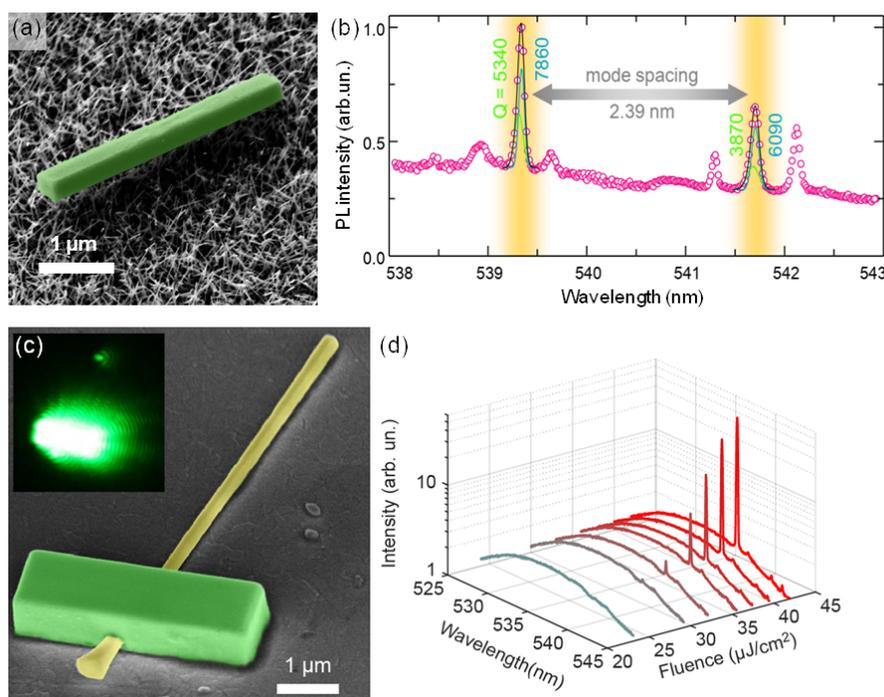
Fig. 1. (a) SEM image of  $CsPbBr_3$  NW on nanostructured ITO substrate. (b) Laser emission of NW with  $9 \mu m$  length. (c) SEM and fluorescent (inset picture) images of GaP nanowaveguide embedded into  $CsPbBr_3$  microcavity. (d) PL intensity collected from GaP end facet versus fluence characteristics.
