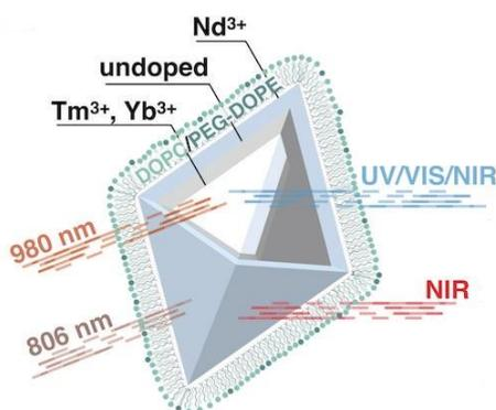
Fig. 1. Schematic representation of the dNPs. The  $\text{LiYF}_4:\text{Tm}^{3+}, \text{Yb}^{3+}$  core absorbs only 980 nm photons and emits UC light from UV to NIR. The core of dNPs is separated by an undoped  $\text{LiYF}_4$  shell #1 from the  $\text{LiYF}_4:\text{Nd}^{3+}$  shell #2 which can be excited by 806 nm irradiation and emit in the NIR spectral region. dNPs are encapsulated in phospholipid micelles, ensuring aqueous colloidal stability and biological applicability.
