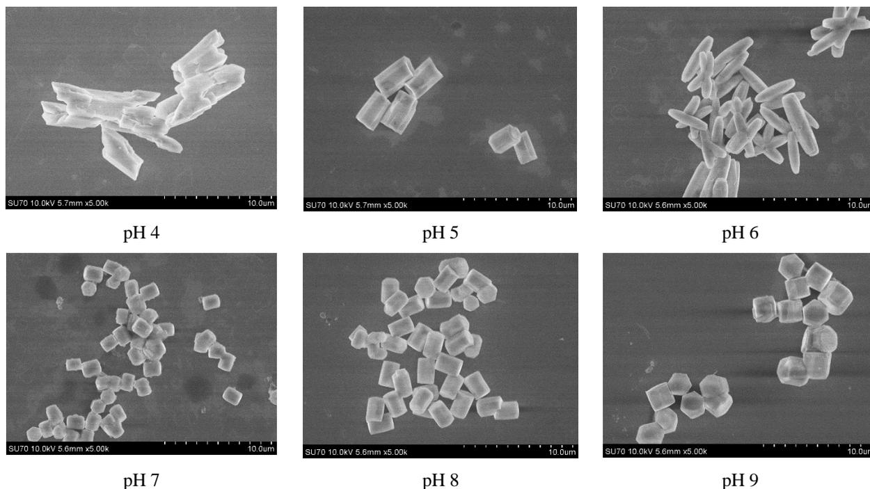
Fig. 1. SEM images of NaYF<sub>4</sub> particles synthesized by hydrothermal synthesis alternating pH values.
