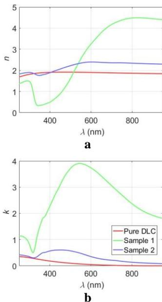
Fig. 1. The dispersion curves of investigated samples: a) refractive index  $n$ ; b) extinction coefficient  $k$ .
