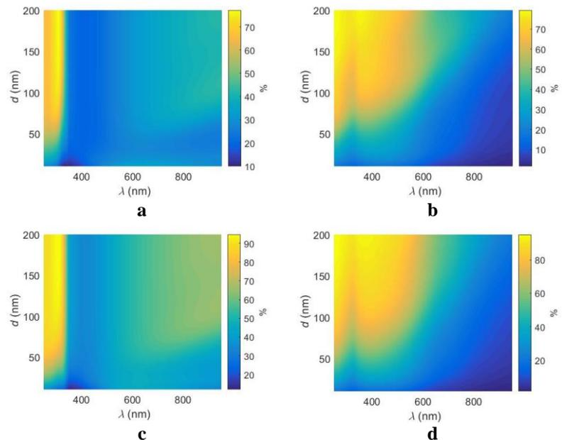
Fig. 2. The modelled absorption results at  $\theta = 45^\circ$ : a) of the sample 1 at  $s$  polarization; b) of the sample 2 at  $s$  polarization; c) of the sample 1 at  $p$  polarization; d) of the sample 2 at  $p$  polarization. Here  $d$  – the thickness of the film,  $\lambda$  – wavelength.
