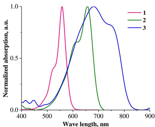
Fig. 2. Absorption spectra for probes 1, 2 and 3
