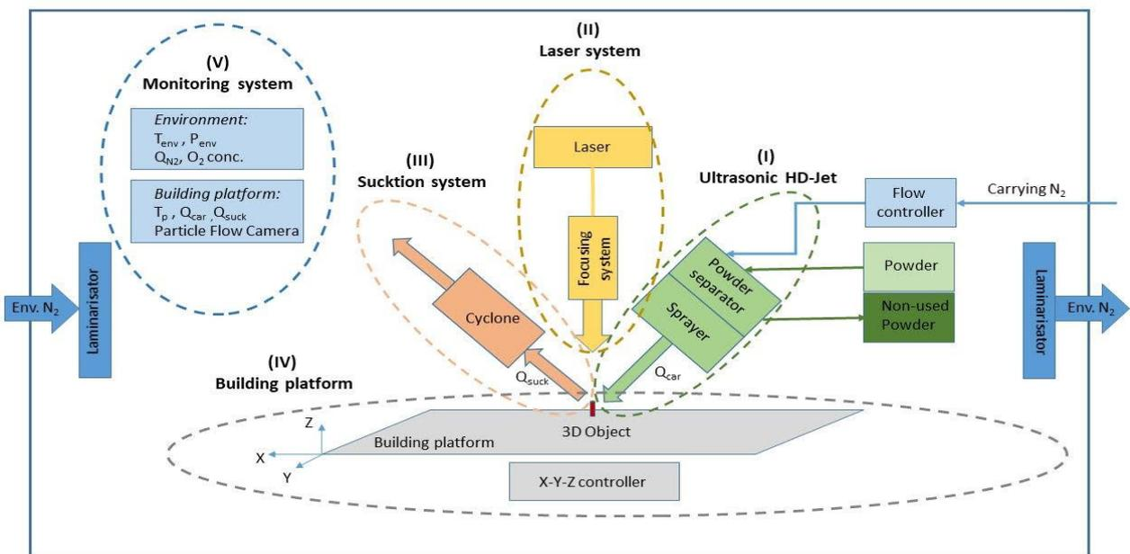
Fig. 1 Technological principle of new LMD system
