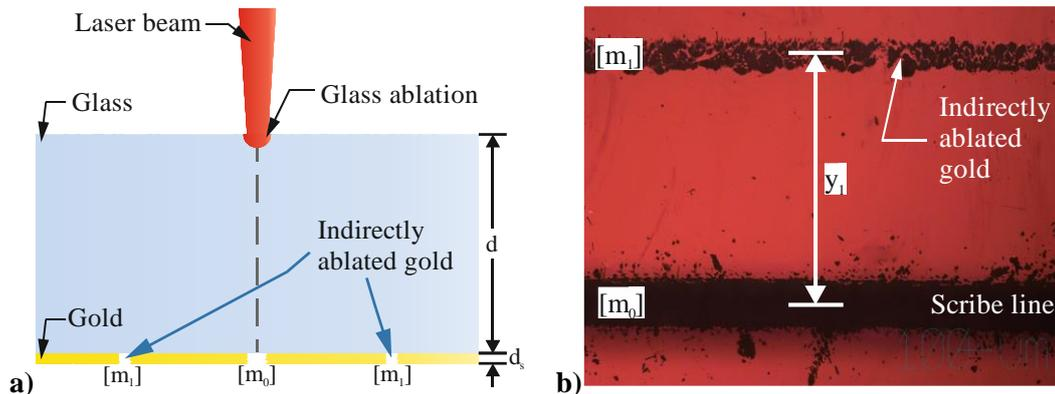
Fig. 1. (a) – Scheme of laser cutting of glass with gold thin film, deposited on the back-side, and ablated areas alongside the scribe line, (b) optical microscope image of the damage alongside the scribe line,  $y_1$  – distance from directly and indirectly ablated lines.
