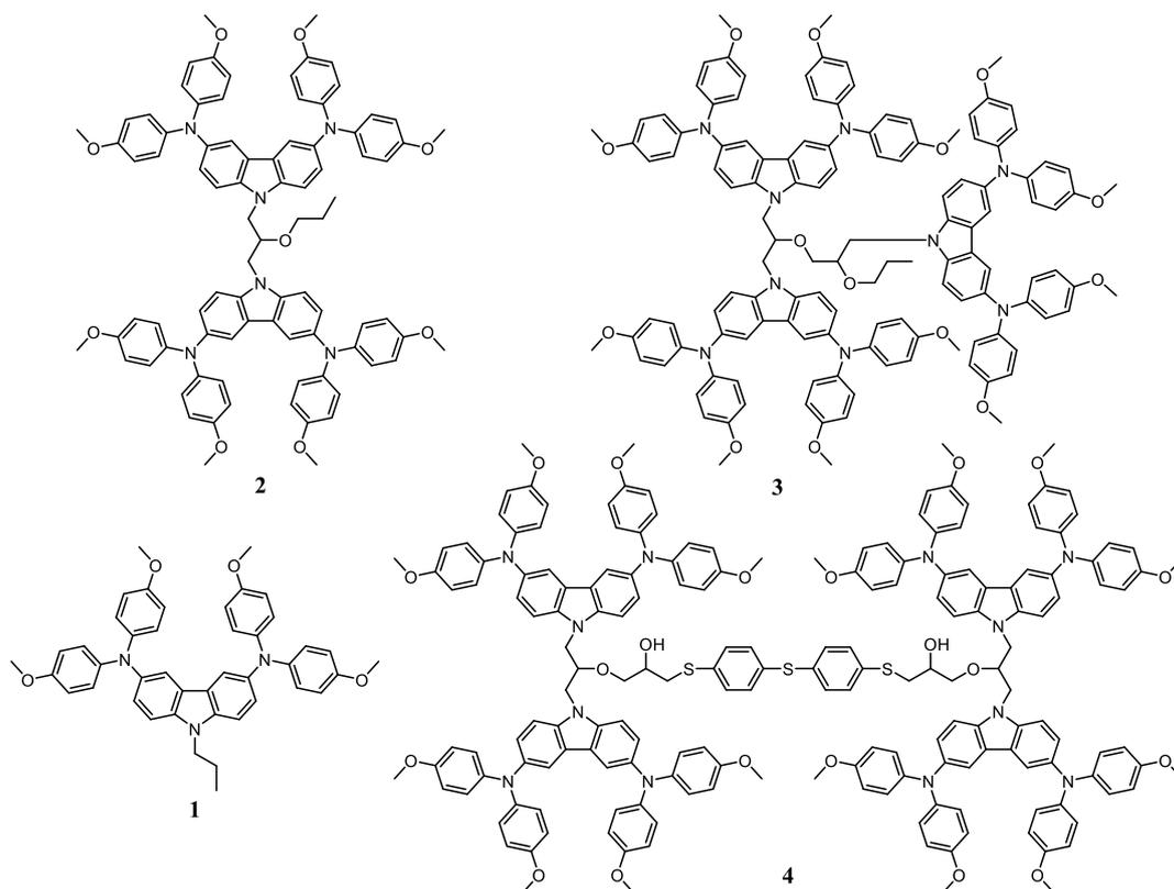
Fig. 1. Structures of synthesized organic semiconductors with carbazolyl chromophores.
