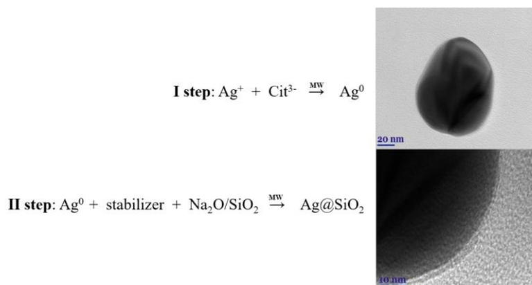
Fig. 1. Synthesis steps and HR-TEM images of Ag and  $\text{Ag}@SiO_2$  nanoparticles.
