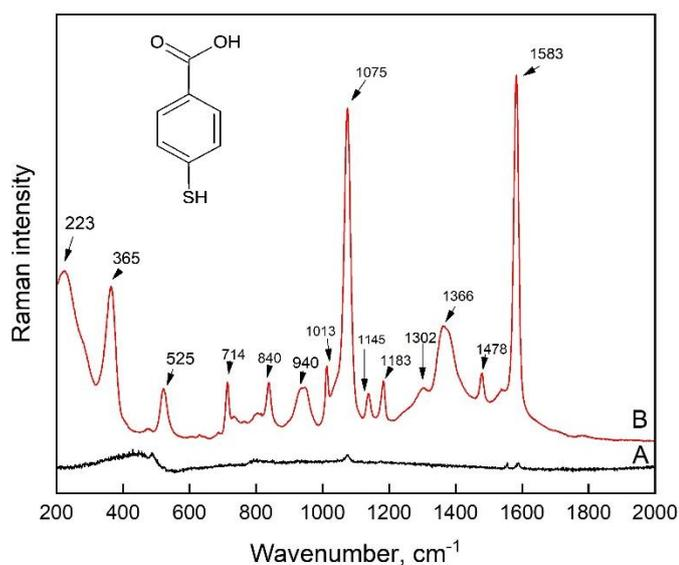
Fig. 2. Raman spectrum of MBA adsorbed on smooth Au surface without nanoparticles (A – black), and SHINERS spectra of MBA with  $\text{Ag}@SiO_2$  nanoparticles (B – red).
