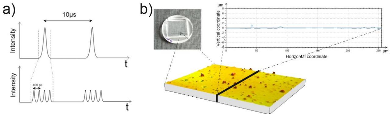
Fig. 1. Femtosecond laser pulse divided into bursts schematic (a), hydrophilic acrylic after polishing using parameters: avg. power = 29 W, scanning velocity = 1 m/s, scanning pitch = 10  $\mu\text{m}$ , number of sub-pulses = 10 (b).
