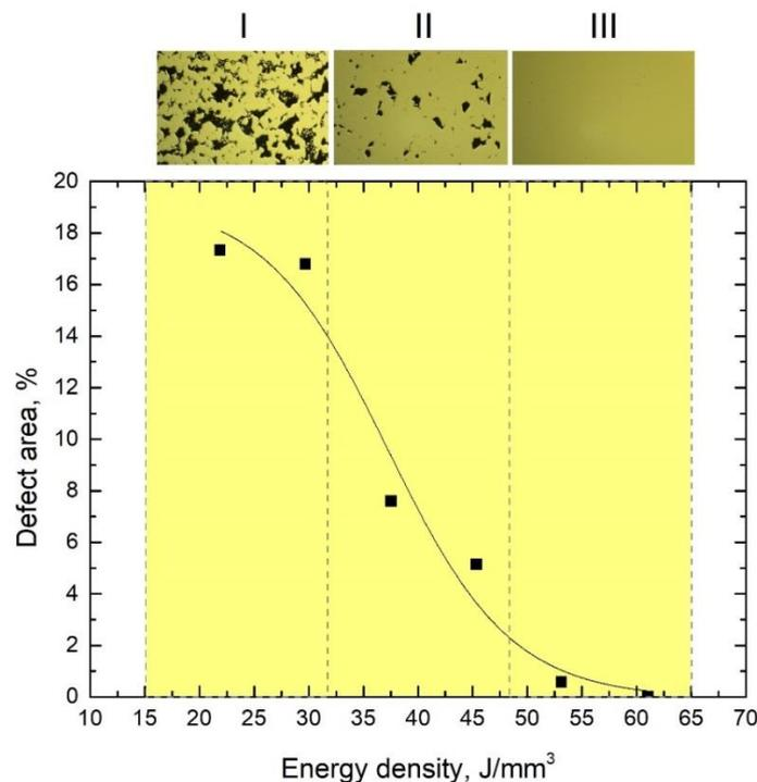
Fig. 1. Microstructural evolution of additively manufactured parts
