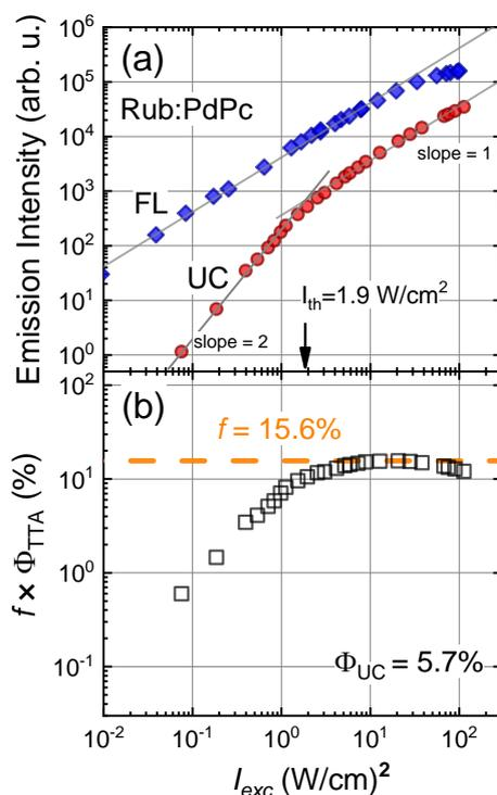
Fig. 1. a) Fluorescence and UC intensities under CW excitation at 485 nm and 730 nm, respectively, as a function of excitation power density for Rub (18mM):PdPc (15 $\mu$ M) in toluene. UC threshold values ( $I_{th}$ ), indicated. b) Excitation dependences of the product [ $f\Phi_{TTA}$ ] of the same system.  $f$  values, indicated.
