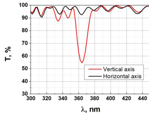
Fig. 2. Transmittance for different directions: vertical axis and horizontal axis.
