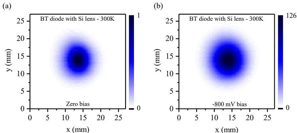
Fig. 1. Images of 150 GHz Gaussian beam recorded with BT diode of 5  $\mu\text{m}$  apex width at different external bias conditions: (a) no bias (b) -0.8 V bias. Detected signal amplitudes are normalised to maximum at zero bias.
