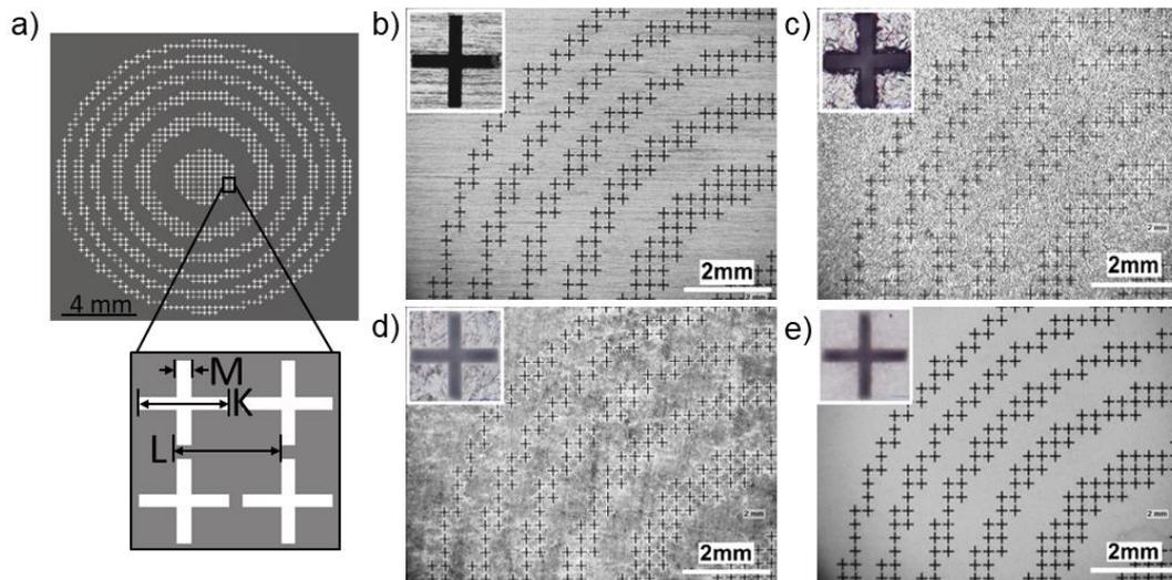
Fig. 1. a) Design of the graphite foil terahertz zone plate for 0.6 THz and geometry of cross-shaped filters ( $M=40 \mu\text{m}$ ,  $K=260 \mu\text{m}$ ,  $L=290 \mu\text{m}$ ). Photos of the quarter of TZP made from different materials: b) metal; c) graphite foil on plastic; d) graphite on paper and e) paper. Insets depicts the shape of cross-shaped aperture element.
