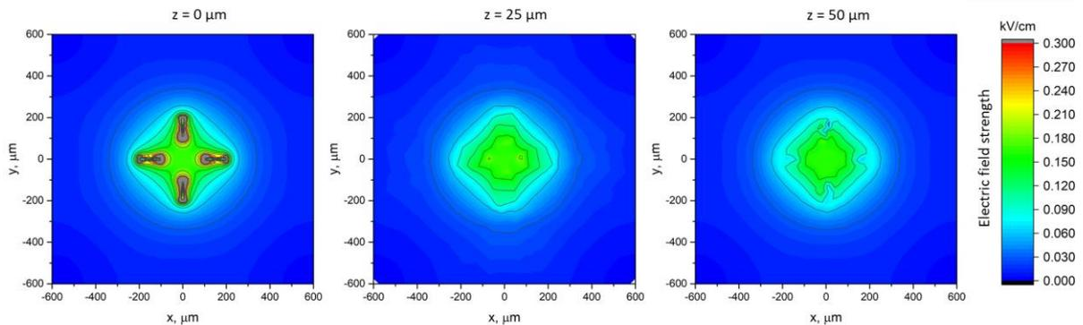
Fig. 1. Electric field distribution of two planar electrodes pairs in XY plane under different height from the electrodes.
