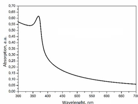
Fig. 1 Absorption spectrum of  $1 \times 10^{-3}$  M ZnO nanoparticles
