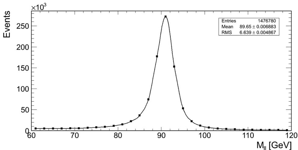
Fig. 1. A histogram shows Z candidate invariant mass distribution, obtained analyzing CMS 2011 collision data using CMS VM.
