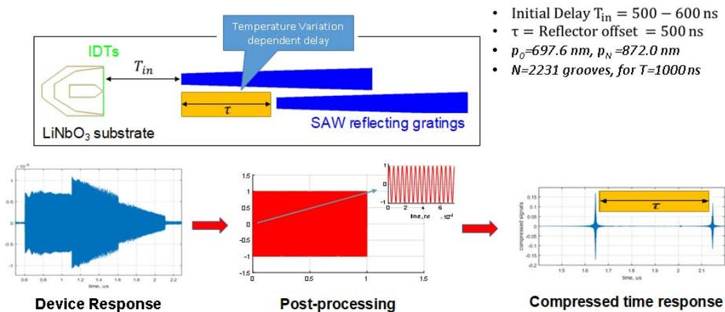
Fig. 1. Operating principle of the SAW sensor. IDTs – interdigital SAW transducers
