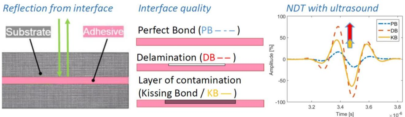
Fig. 1. Schematic of single lap joint on the left. Different bonding (interface) quality schematics at the centre. The A-scan ultrasonic inspection of different interface qualities (semi analytical finite-element numerical study results- first interface time window) on the right.
