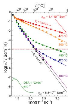
Fig. 1. Conductivity in function of temperature [3]. Black colour refers to data obtained during heating, whereas coloured marks represent values obtained in cooling after heating to various temperatures. Brown line stands for conductivity of crystalline material and the green one represents DTA curve for 1°C/min for comparison.
