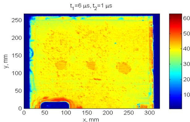
Fig. 1. C-scan of the inspection of dissimilar material joints in immersion pulse echo mode.
