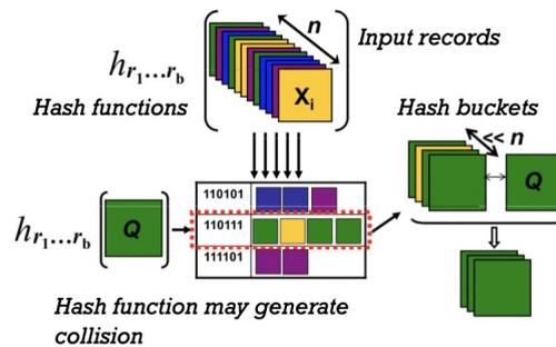
Fig. 1. Locality-Sensitive Hashing algorithm
