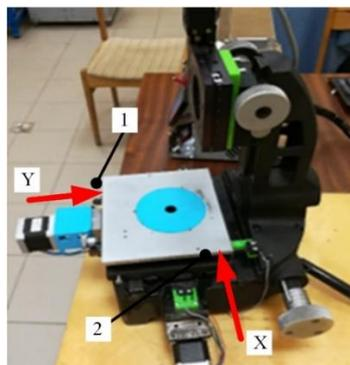
Fig. 1 Micro-electromechanical positioning system: 1, 2 – sensors mounting places
