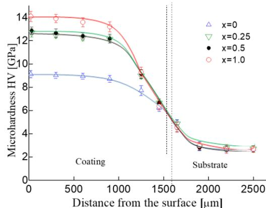
Fig. 2. Hardness of  $\text{AlNiCoFeCrTiB}_x$  HEA coatings received from electron beam cladding.
