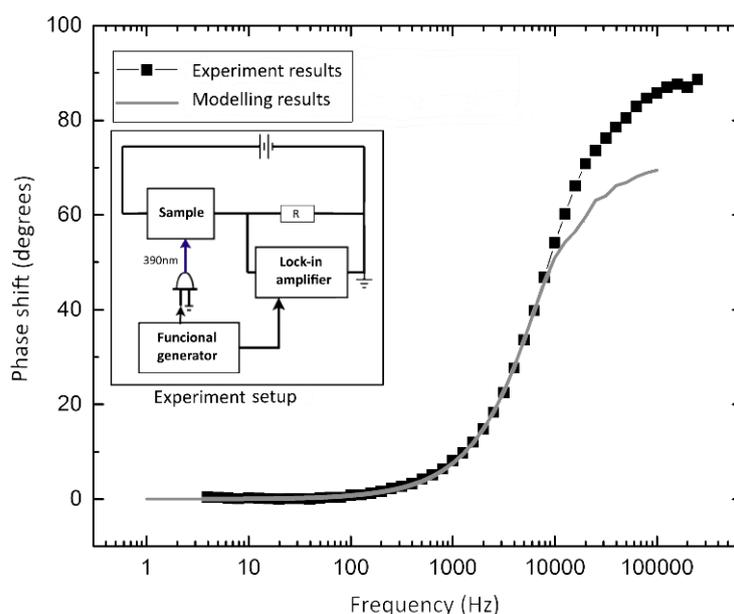
Fig. 1. Experiment results comparison with modelling results and the experiment setup (inset).
