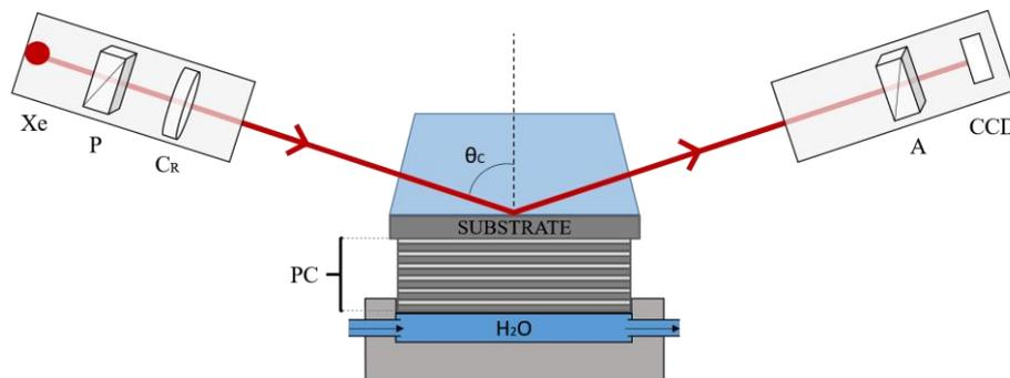
Fig. 1. TIRE schematic used for BSW generating. Components of ellipsometer: LS – light source, P – polarizer, CR – rotating compensator, A – analyzer, CCD detector.
