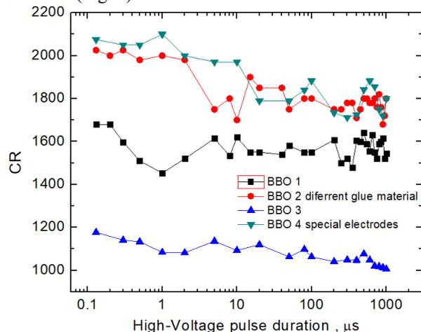
Fig. 2. Contrast ratio (1/CR) dependence of BBO Pockels cells on high-voltage control pulse duration.
