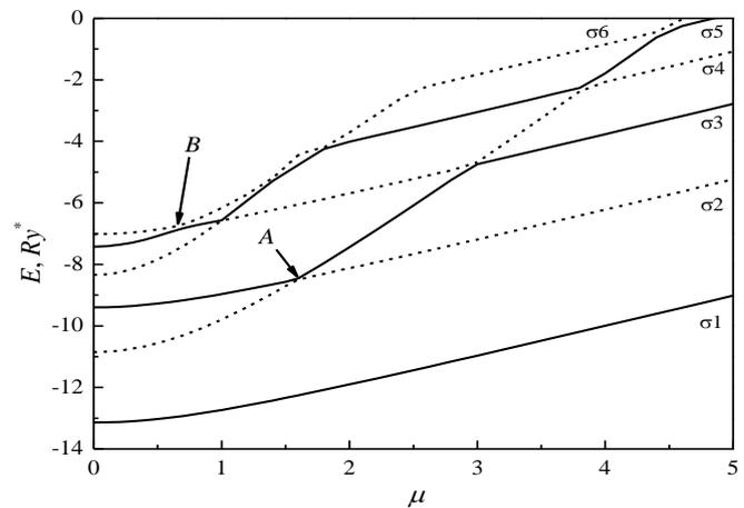
Fig. 1. Ground and lowest excited state energies of electrically defined quantum dot as functions of magnetic field value. The calculation was carried out for gate diameter  $d = 6a^*$  and gate potential  $\Phi_0 = 20 Ry^*/e$ .
