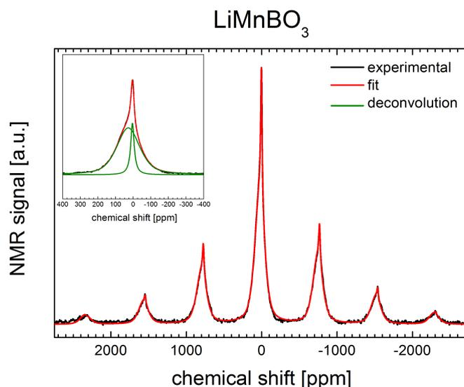
Fig. 1. Experimental (black line) and best-fit simulated (red line) 1D  $^7\text{Li}$  MAS NMR spectrum of the initial glass (black line) at 1.9 T with a MAS frequency of 30 kHz. The inset shows an expansion of the central transition. The simulated  $^7\text{Li}$  spectrum is the sum of two distinct lineshapes (displayed as olive lines in the inset).
