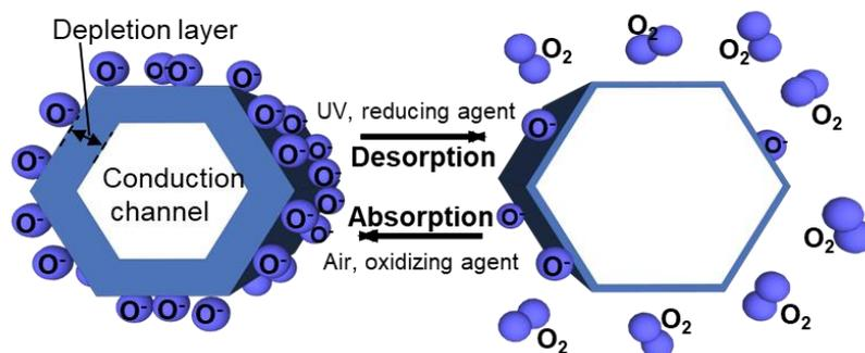
Fig. 1. Principle of ZnO nanowire chemoresistive sensing based on the depletion layer width change with absorption-desorption of oxygen
