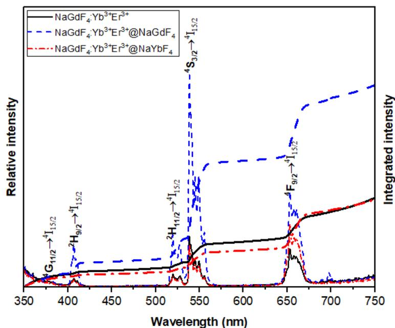
Fig. 1. Emission intensity comparison of NaGdF<sub>4</sub>:Yb<sup>3+</sup>,Er<sup>3+</sup>, NaGdF<sub>4</sub>:Yb<sup>3+</sup>,Er<sup>3+</sup>@NaGdF<sub>4</sub> and NaGdF<sub>4</sub>:Yb<sup>3+</sup>,Er<sup>3+</sup>@NaYbF<sub>4</sub> nanoparticles. Core-shell nanoparticles were synthesized at 310 °C, 90 min.
