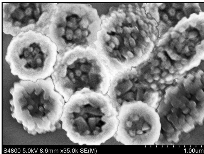
Fig. 1. SEM-image of the nanocoatings' consisting of one layer of large nanostructured porous fractal aggregates nC<sub>60</sub>. The image was obtained on the surface of the mica substrate after complete evaporation of the solvent.
