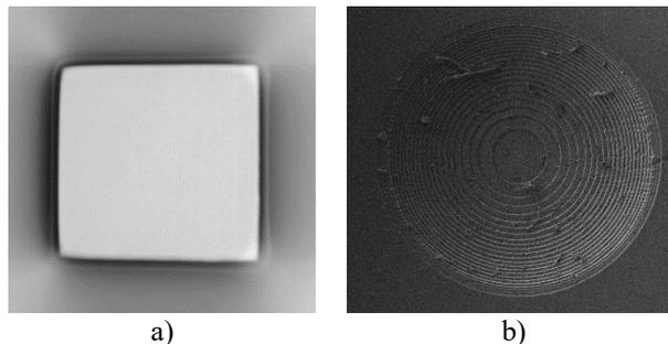
Fig. 1. a) The view of square structure from its bottom, after 60 min of etching and 2 second of melting. b) The view of spherical lens after etching and melting. ( $E = 200$  nJ,  $dy = 2,5$  μm,  $v = 5$  mm/s).
