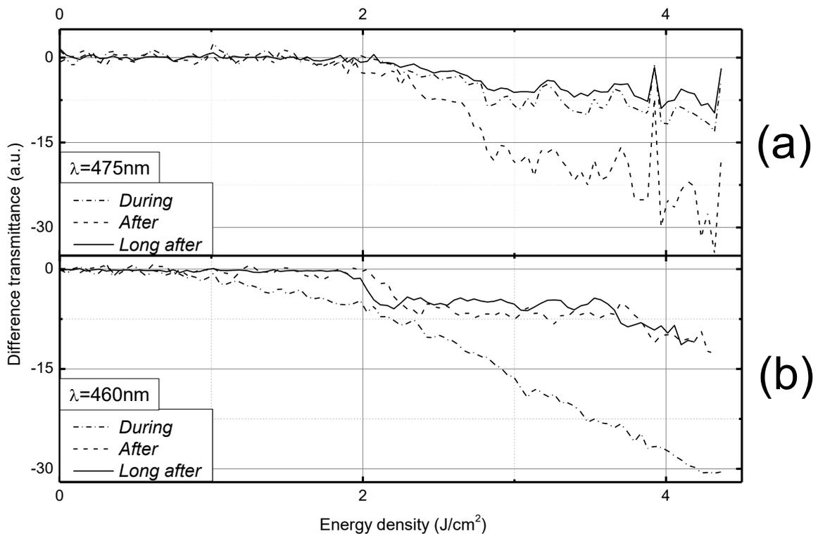
Fig. 1. Difference transmittance dependence on energy density of (a) borosilicate glass at 475nm; (b) titanium dioxide dielectric coating at 460nm.
