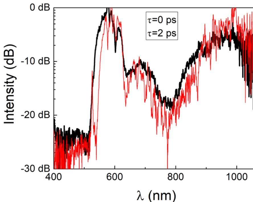
Fig. 1. Supercontinuum spectra: black curve – temporal delay between pulses in the burst is zero; red curve – two picoseconds.
