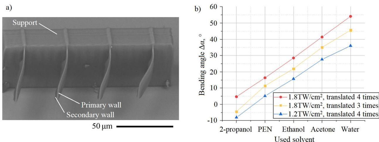
Fig. 1. SEM image of a structure with bipolymeric walls. Support and primary walls are fabricated out of SZ2080, secondary walls – out of PEG-DA-575 (a). Bending angle dependence on secondary walls fabrication parameters and solvent (b). (PEN - 4-methyl-2-pentanone)
