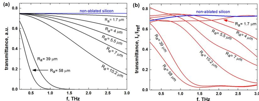
Fig. 2. Transmittance of nanosecond laser ablated silicon with various surface roughness in 0.2 – 3.0 THz frequency range (b), compared with theoretical scattering model (a).
