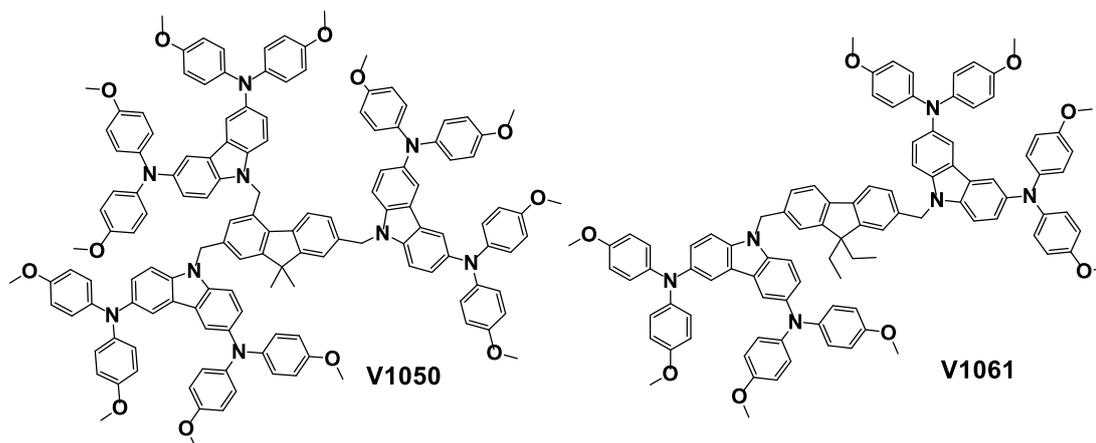
**Figure 1.** Structures of fluorene-based HTMs **V1050** and **V1061**.
