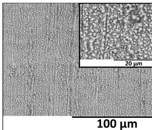
Fig. 1. SEM image of  $\text{MoS}_{2-n}\text{Se}_n$  film (inset is a high magnification image), electrodeposited at  $-1.0$  V vs Ag/AgCl for 600 s from the electrolyte containing 25 mM of  $\text{MoS}_3\text{Se}$ .
