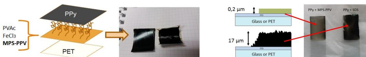
Fig. 1. MPS-PPV application ideas for PPy composite layer and electrochemically synthesized PPy on ITO.
