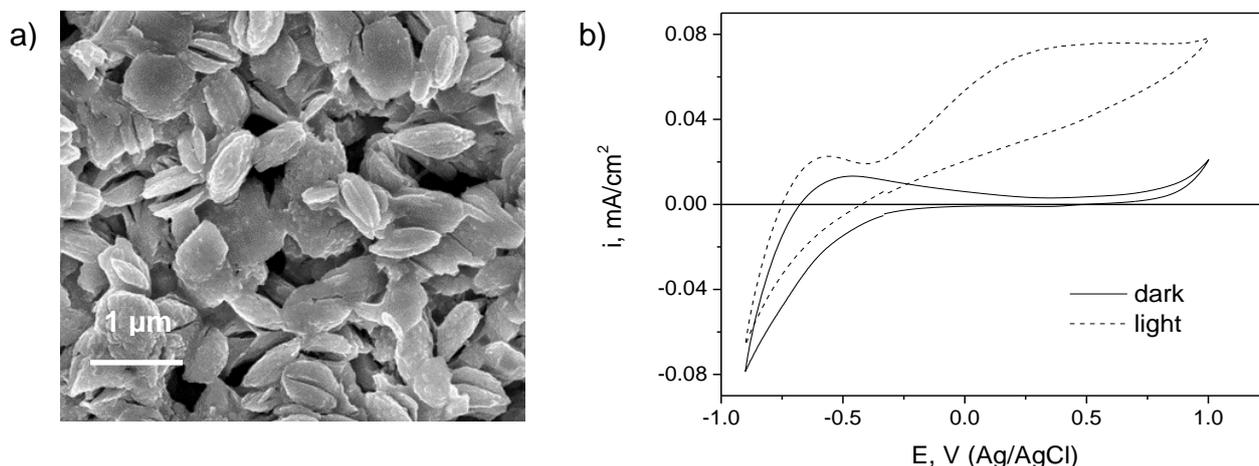
Fig. 1. a) SEM image of sol-gel derived WO<sub>3</sub> film, b) cyclic voltammograms of FTO/WO<sub>3</sub> photoelectrode in 0.5 M NaCl + 1.0 M KOH solution in dark and under illumination (100 mW cm<sup>-2</sup>) run at 50 mV/s
