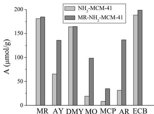
Fig. Removal of dye pollutants by NH<sub>2</sub>-MCM-41 (light gray) and MR-NH<sub>2</sub>-MCM-41 (dark gray) from phosphate buffer solutions (pH 4.8) with initial concentrations of dyes equal to 0.2 mmol/l.
