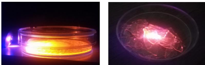
Figure 1. Matrix doped with: left -  $\text{Sm}_2\text{O}_3$ , right:  $\text{Eu}_2\text{O}_3$ .
