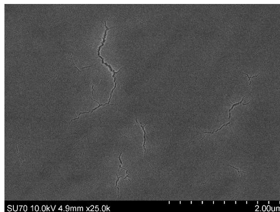
Figure 2. Y<sub>0,06</sub>Zr<sub>0,93</sub>Mg<sub>0,01</sub>O<sub>1,96</sub> coating on titanium substrate
