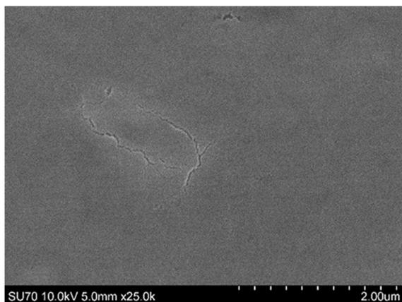
Figure 1. Y<sub>0,06</sub>Zr<sub>0,93</sub>Ca<sub>0,01</sub>O<sub>1,96</sub> coating on titanium substrate
