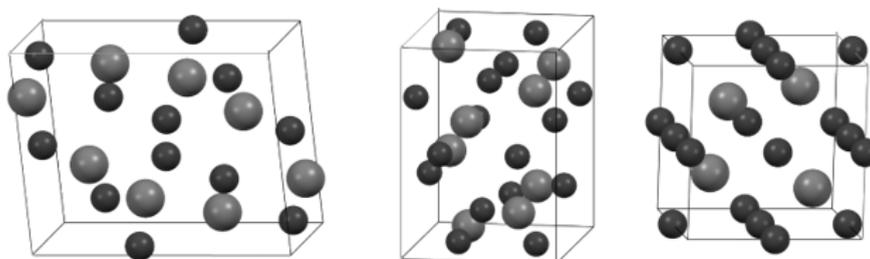
Fig. 1. Unit cells of the most important phases of bismuth (III) oxide (from left to right): ( $P2_1/C$ ) monoclinic ( $\alpha$ ); ( $P42_1C$ ) tetragonal ( $\beta$ ); ( $Pn-3m$ ) fluorite-type fcc ( $\delta$ ), generated by Mercury software [2] from CIFs no. 1010004, 1545547, 1010311, respectively.
