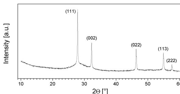
Fig. 2. Room temperature XRD pattern of as-synthesized material. Miller indexes of  $\delta$ - $\text{Bi}_2\text{O}_3$  phase, assigned to experimental diffraction lines, prove that the fcc phase was obtained.
