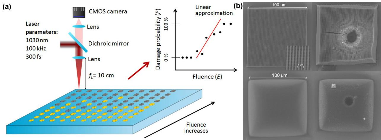
**Fig. 1. (a)** Scheme of LIDT measurement experiment. **(b)** Formed polymeric bulk and woodpile structures before and after LIDT experiment. Top left woodpile before LIDT testing, top right woodpile after LIDT testing, bottom left bulk before LIDT experiment, bottom right bulk after LIDT experiment.
