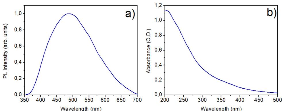
Fig. 1. Photoluminescence (a) and Absorption (b) spectra of GOQDs water solution.
