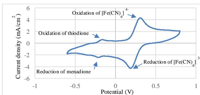
Fig. 1. The cyclic voltamperogram measured with a carbon electrode modified by yeast in phosphate-acetate buffer solution with 4.21 mM potassium ferricyanide, 80.5mM glucose and 512  $\mu$ M menadione. Scan rate 0.1 V/s and the potential range from -0.6 V to 0.6 V. Reduction and oxidation peaks of menadione appears at -0.2 V and - 0.16 V; oxidation and reduction peaks of  $K_3[Fe(CN)_6]$  appears at 0.2 V and 0.3 V, respectively.
